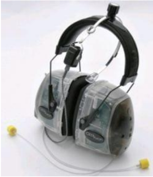
Figure 1. KUDUwave 5000 audiometer (GeoAxon, South Africa) Type 2 clinical audiometer. Hardware encapsulated in the earcups with USB power from notebook and USB response button. Insert earphones covered by circumaural earcups for additional passive attenuation and microphones on the outside of each earcup for active monitoring of environmental noise levels during testing.
