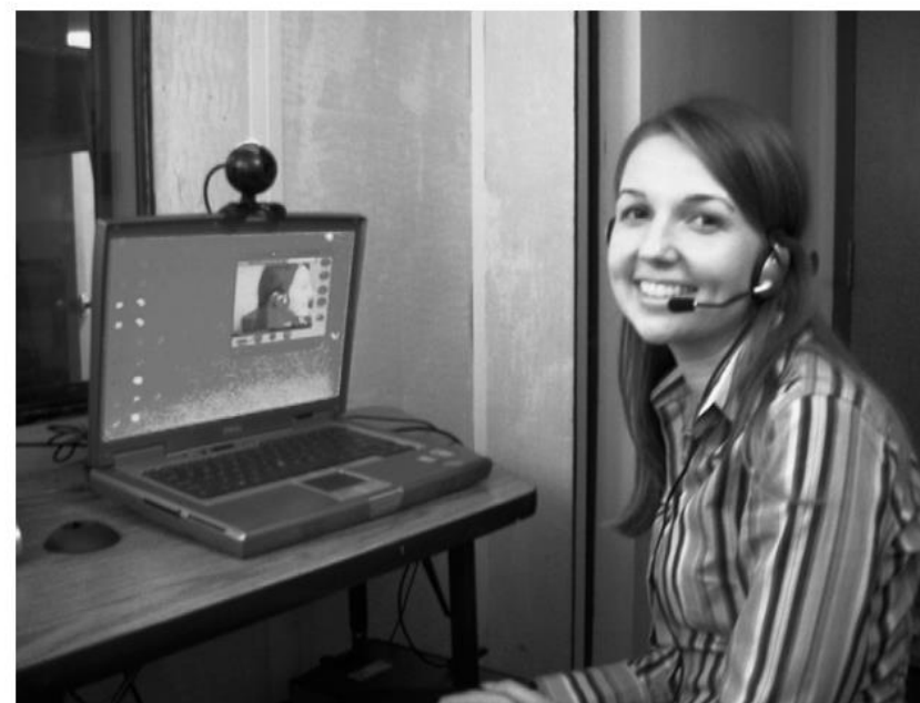
Fig. 2. The clinician equipment configuration for an audiologist administering telehealth services. Note only a computer (with remote computing software) and a video system (either web cam or dedicated video) are required at the clinician site.
