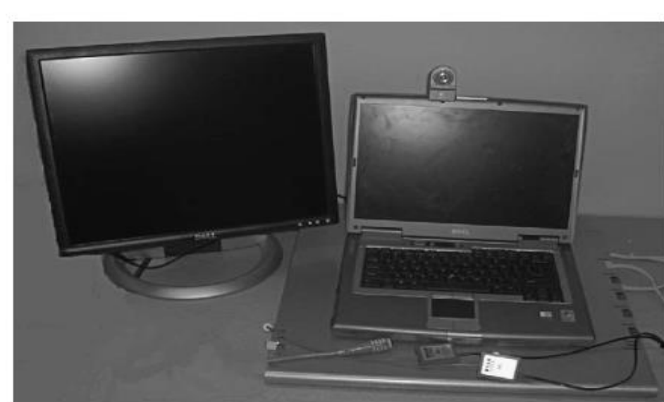
Figure 1 The computerized audiometry equipment at the patient's site included the audiometer unit (positioned under the laptop computer) and an auxiliary monitor. The audiometer headphones and a client handheld switch are
