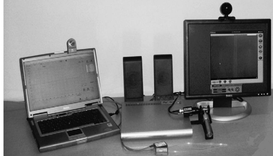
Fig. 3. Equipment required at the patient site. For remote computing purposes, a computer, Web camera or dedicated camera, computerized audiometric equipment (an audiometer is pictured), video-otoscopy, immittance (not shown), and a LAN connection would permit basic teleaudiology services.
